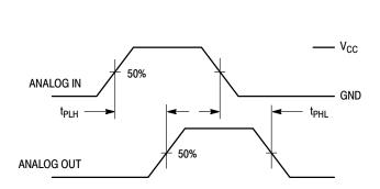
Figure 10. Propagation Delay, Analog In to Analog
