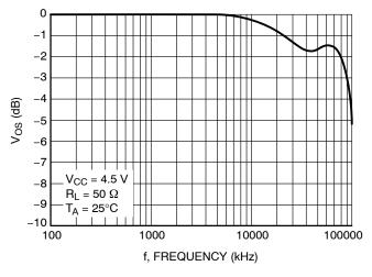
Figure 5. Typical Switch Frequency Response
