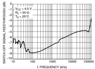
Figure 6. Typical Switch OFF Signal Feedthrough vs Frequency
