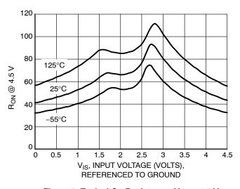
Figure 3. Typical On Resistance,  $V_{CC} = 4.5 \text{ V}$
