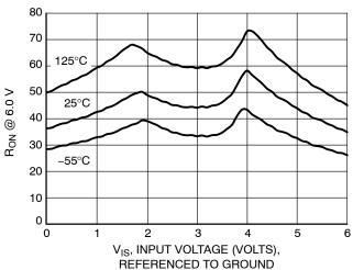
Figure 4. Typical On Resistance, V<sub>CC</sub> = 6.0 V
