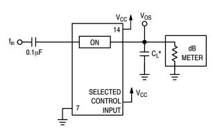
\*Includes all probe and jig capacitance.
