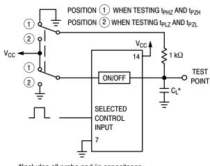
\*Includes all probe and jig capacitance.
