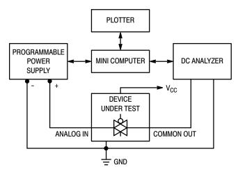
Figure 7. On Resistance Test Setup
