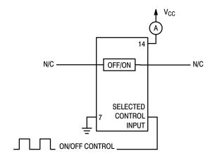
Figure 14. Power Dissipation Capacitance
