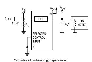
Figure 16. OFF Channel Feedthrough Isolation
